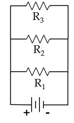
Questions 6 and 7 refer to the following: The diagram to the right represents an electric circuit consisting of four resistors and a 12-volt battery.
