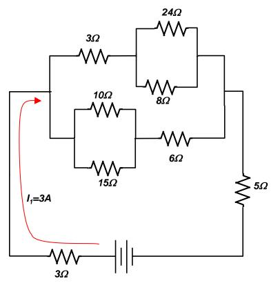
b) Find the equivalent resistance, Req, of the circuit
