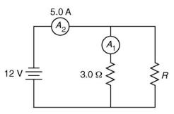
11) Determine the equivalent resistance of the circuit shown.
