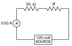
9) Calculate the equivalent resistance of the circuit shown.
